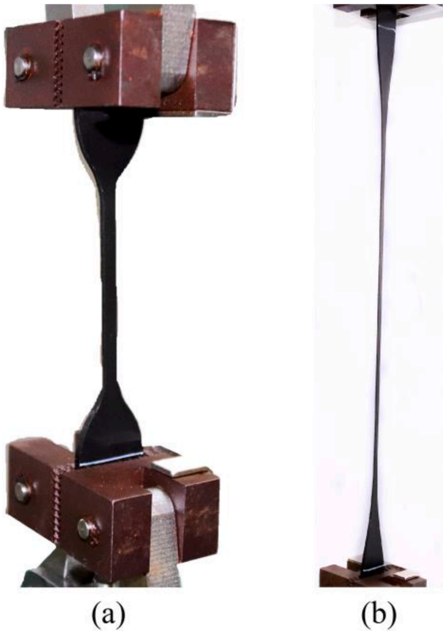
Fig. 3. Dumbbell-shaped sample under quasi-static uniaxial tension: (a) initial state and (b) highly stretched.
