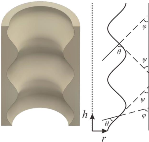
**FIG. 2.** The apparent contact angle  $\phi$  on the undulated inner surface of a circular tube gradually changes with tube position  $h$ . The origin of the cylindrical coordinates is placed at the tube center ( $r=0$  and  $z=0$ ).
