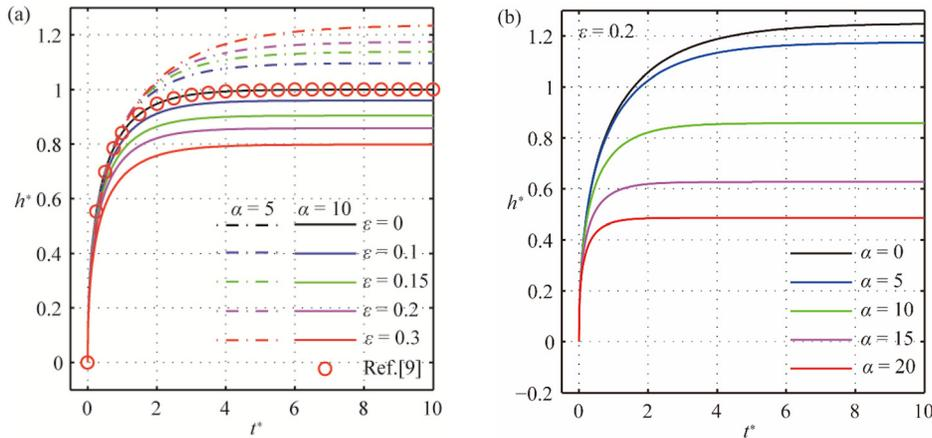
FIG. 3. Dynamic rising in the small-inertia case ( $\Omega = 100, \phi = \pi/2$ ) for selected undulation amplitudes and wave numbers: (a)  $\alpha = 5$  and  $10$  and (b)  $\varepsilon = 0.2$  (from top,  $\alpha = 0, 5, 10, 15,$  and  $20$ ).
