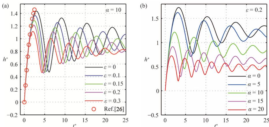
FIG. 6. Dynamic fluid-rise in the small-viscosity case ( $\Omega = 0.1$ ,  $\phi = \pi/2$ ) for selected undulation amplitudes and wave numbers: (a)  $\alpha = 10$  (from top,  $\varepsilon = 0, 0.05, 0.1, 0.2$ , and  $0.3$ ) and (b)  $\varepsilon = 0.2$  (from top,  $\alpha = 0, 5, 10, 15$ , and  $20$ ).
