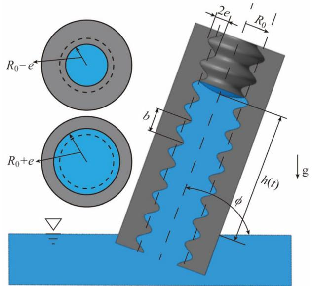
FIG. 1. Capillary rise in a circular tube with a cosinoidally undulated inner wall.  $R_0$  is the mean radius of the tube,  $e$  is the undulation amplitude,  $b$  is the undulation wavelength, and  $\phi$  ( $0 \leq \phi \leq \pi/2$ ) is the orientation angle of the tube.
