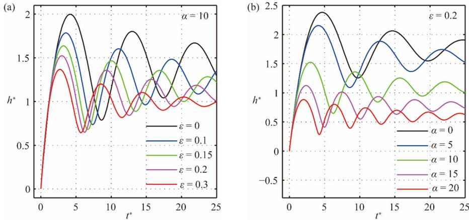
**FIG. 7.** Dynamic fluid-rise in small-viscosity case ( $\Omega = 0.1$ ,  $\phi = \pi/4$ ) for selected undulation amplitudes and wave numbers: (a)  $\alpha = 10$  (from top,  $\varepsilon = 0, 0.05, 0.1, 0.2$ , and  $0.3$ ) and (b)  $\varepsilon = 0.2$  (from top,  $\alpha = 0, 5, 10, 15$ , and  $20$ ).
