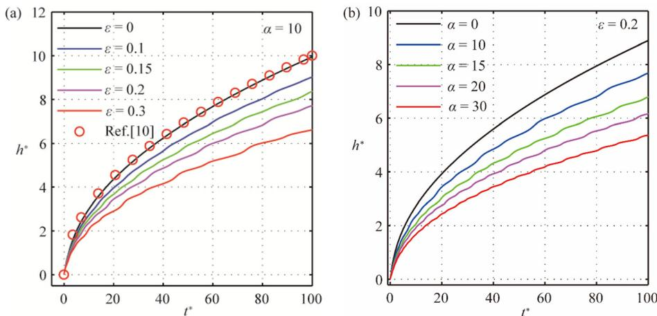
**FIG. 8.** Dynamic fluid-rise for the case of negligible gravity ( $\Omega = 100$ ) and for selected undulation amplitudes and wave numbers: (a)  $\alpha = 10$  (from top,  $\varepsilon = 0, 0.05, 0.1, 0.2$ , and  $0.3$ ) and (b)  $\varepsilon = 0.2$  (from top,  $\alpha = 0, 5, 10, 15$ , and  $20$ ).
