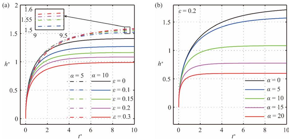
FIG. 4. Dynamic fluid rise in the small-inertia case ( $\Omega = 100, \phi = \pi/4$ ) for selected undulation amplitudes and wave numbers: (a)  $\alpha = 5$  and  $10$ , and (b)  $\varepsilon = 0.2$  (from top,  $\alpha = 0, 5, 10, 15,$  and  $20$ ).
