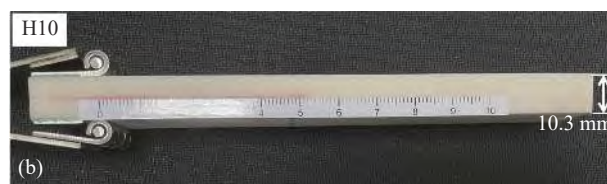
Fig. 4 (a) DCB specimen with interlaminar pre-crack; (b) DCB specimen with pasted scale and loaded hinge
