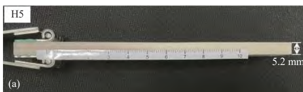
Fig. 4 (a) DCB specimen with interlaminar pre-crack; (b) DCB specimen with pasted scale and loaded hinge
