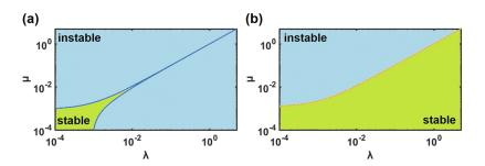
**FIG. 4.** Phase diagram of stability: (a) first mode and (b) second mode.
