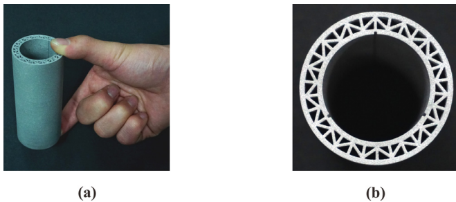
Fig. 3. Sandwich-walled cylinder manufactured via 3D-printing: (a) holistic view; (b) top view.
